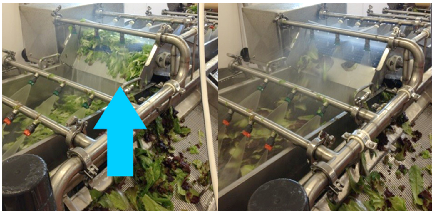
Figure 1. Lettuce cultivar with a flat leaf structure tends to clog processing equipment (left), whereas cultivars with loft pass through the equipment more easily (right).
